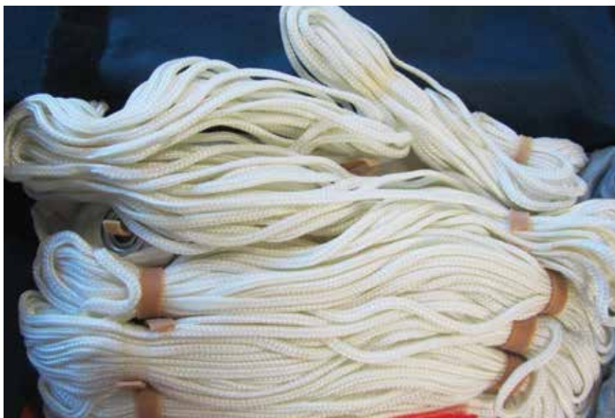
Brittle, broken rubber bands holding the lines in place are a sign of long-term damage and should be replaced.
