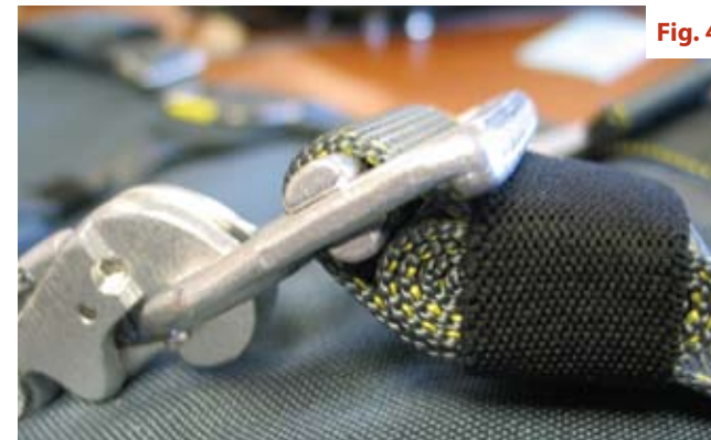
Figures 3 and 4: Be sure excess webbing is not stowed too close to adapters as they could cause the adapter to loosen during deployment.
