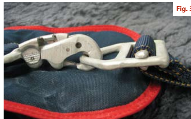
Figures 3 and 4: Be sure excess webbing is not stowed too close to adapters as they could cause the adapter to loosen during deployment.
